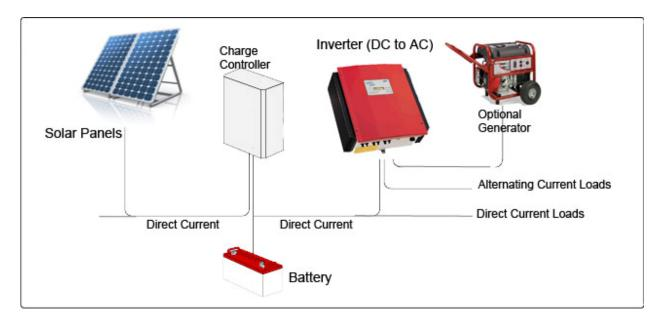
In some cases, where it is important that power is always available, some stand alone systems, known as PV-hybrid systems or island systems, may also have another source of power such as a wind turbine, bio-fuel or a diesel generator.
